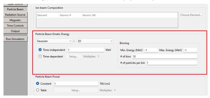
The distribution option (e.g. Gaussian) appears in the first combo-box. For each distribution option (except Tabulated), the distribution is defined by one or more parameters. The parameter being specified appears in the second combo-box. Each parameter can be either time-independent or time-dependent.
